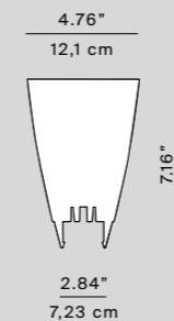
Polycarbonate diffuser for halogen
